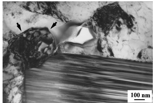
Figure 4 TEM detail of recrystallization in a whisker corner (marked with arrow).
